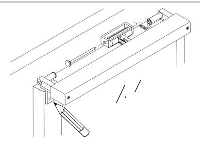
Mount drive brackets. With a wing projection of less than 15mm underfill drive brackets with enclosed distance plates (m, n) up to at least 15mm.
