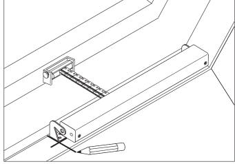
**7** Put drive brackets against marking, and mark borings, pilot-drill if necessary. Screw down lefthand and righthand drive bracket.
