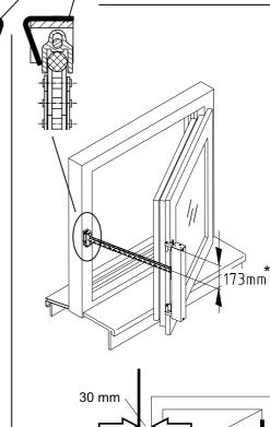
Minimum space required to the left side of the window frame: 30 mm.
