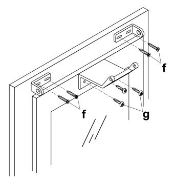
4 Mount chain drive in drive brackets with bearing screws.
