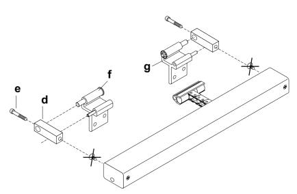
Mount chain tail-piece with bracket pin in frame bracket. Safeguard the bracket pin with the cotter pin.
