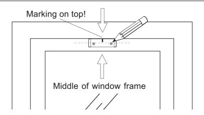
Put template against lower edge of window frame, mark borings for drive brackets (d+e), pilot-drill, if necessary.
