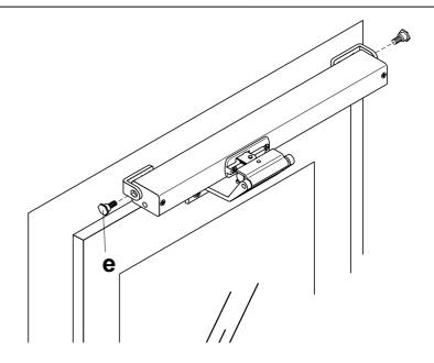
Mount chain tail-piece with bracket pin in wing bracket. Safeguard bracket pin with cotter pin.
