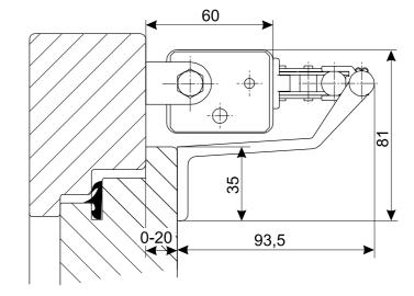
Mark borings for drive brackets (d), according to stroke, with enclosed template.
