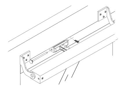
5 Mount chain drive in drive brackets with bearing screws.
