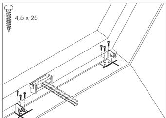
Mount drive in drive brackets with the screw type bearings.
