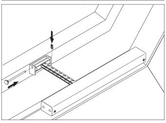
6 Screw-in handtight screw type bearings, hang up lefthand and righthand drive bracket, and mark position of brackets.
