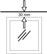
Minimum space required on window frame: 30 mm.
