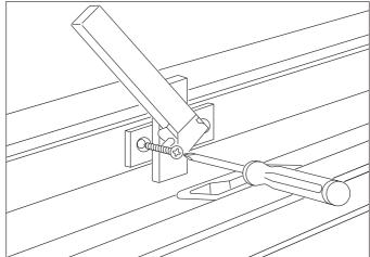
**GGL / GGU / VL:** Fasten wing bracket at window wing with countersunk screws.
